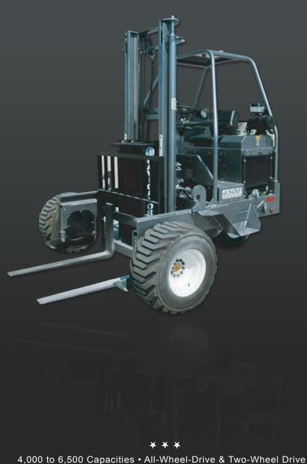
Nav-Reach Extension Mechanism • Water Cooled Diesel, All-Terrain, Truck-Mounted Forklifts
