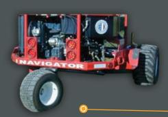
Optional Jumbo Caster assembly provides increased flotation to the rear of the Rt-4000
