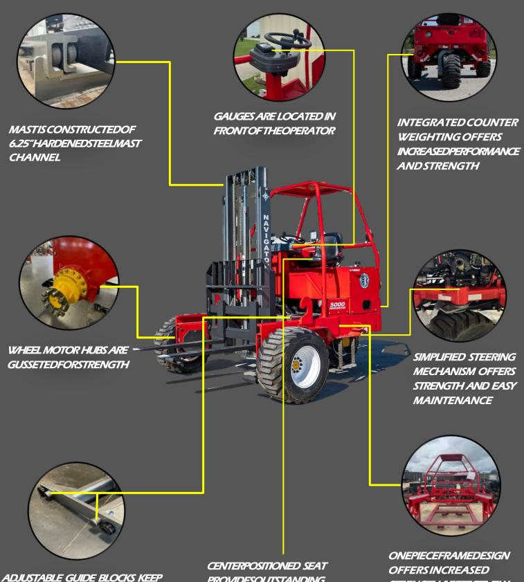
ADJUSTABLE GUIDE BLOCKS KEEP SLIDE CARRAIGE STRAIGHT IN THE FRAME CENTERPOSITIONED SEAT PROVIDESOUTSTANDING COMFORT, SAFETY AND VISION
